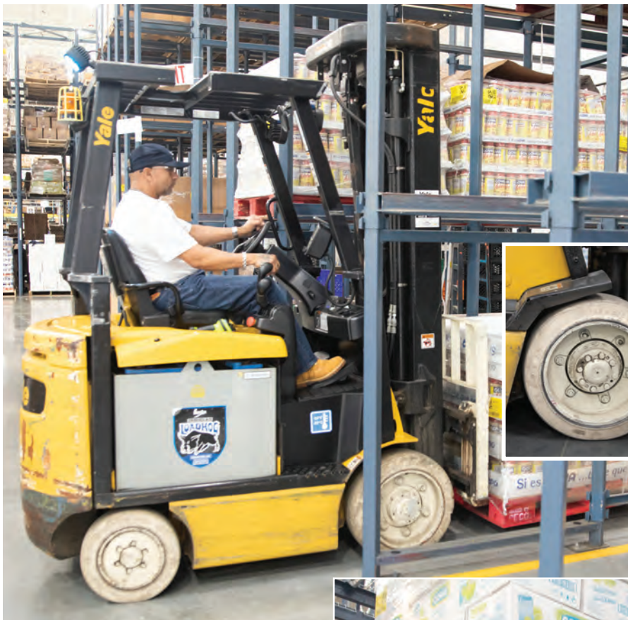
The Goya Spec truck (top left) was modified to work with drive-in racks. Very narrow aisle lift trucks (bottom right) operate in the slow-moving goods area.
