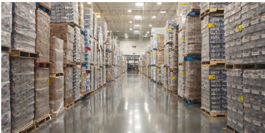
The Jersey City facility relies on a number of different storage strategies, ranging from floor storage to nine-pallet-high narrow aisle storage.
