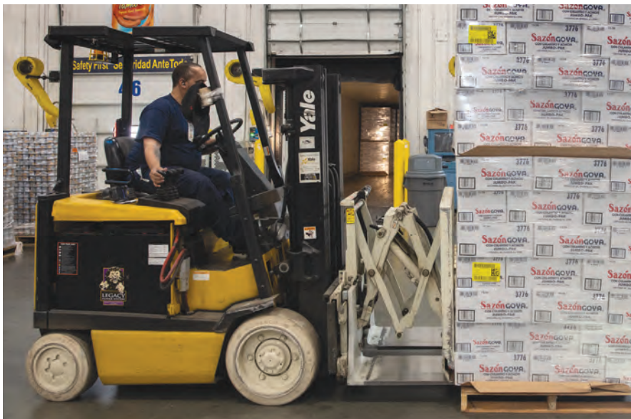
Special attachments are used for slip sheet handling.
