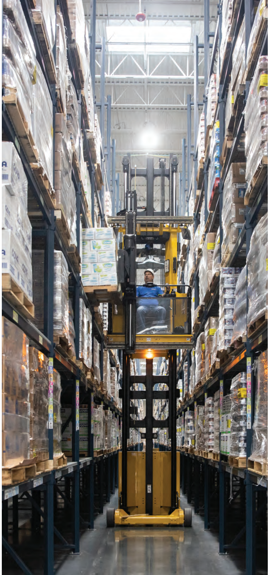
A narrow aisle turret truck puts away a pallet in the VNA storage area.
