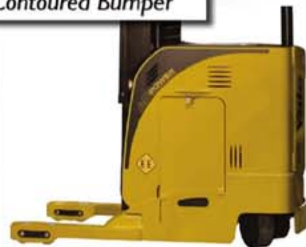
UL 'EE' Construction
